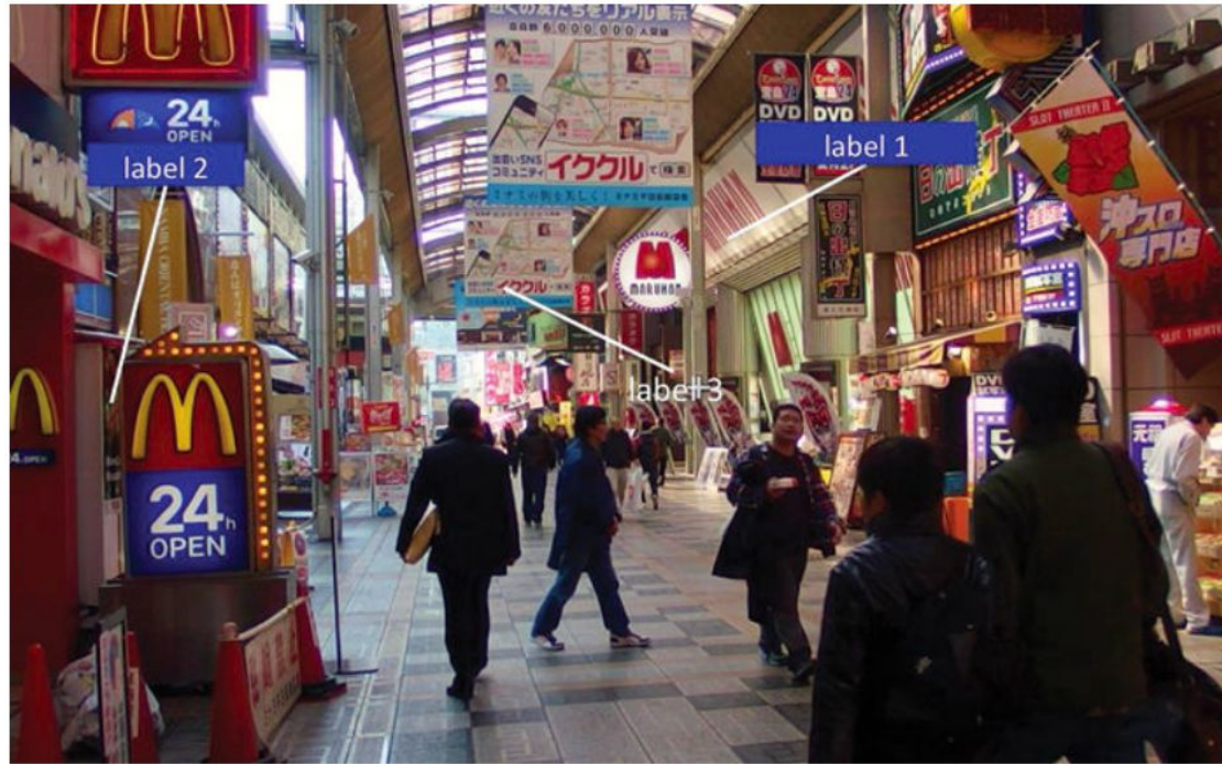
Figure 9.10 Legibility with different backgrounds in augmented reality. This mockup image shows several frequently occurring issues: the leader line of label 1 (right) is difficult to see due to the light background, whereas label 2 (left) can be overlooked due to the low color contrast with the blue sign behind and above it. Label 3 can barely be read, as the label does not have a background color. While this reduces occlusion, in this case legibility is low due to the low contrast and pattern interferences of the background.
